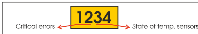
Figure 6.1: Division of heat pump faults and states
